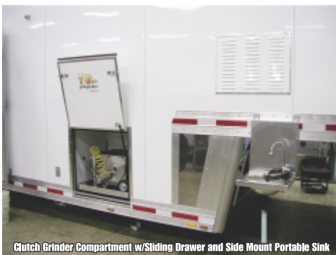
Clutch Grinder Compartment w/Sliding Drawer and Side Mount Portable Sink
